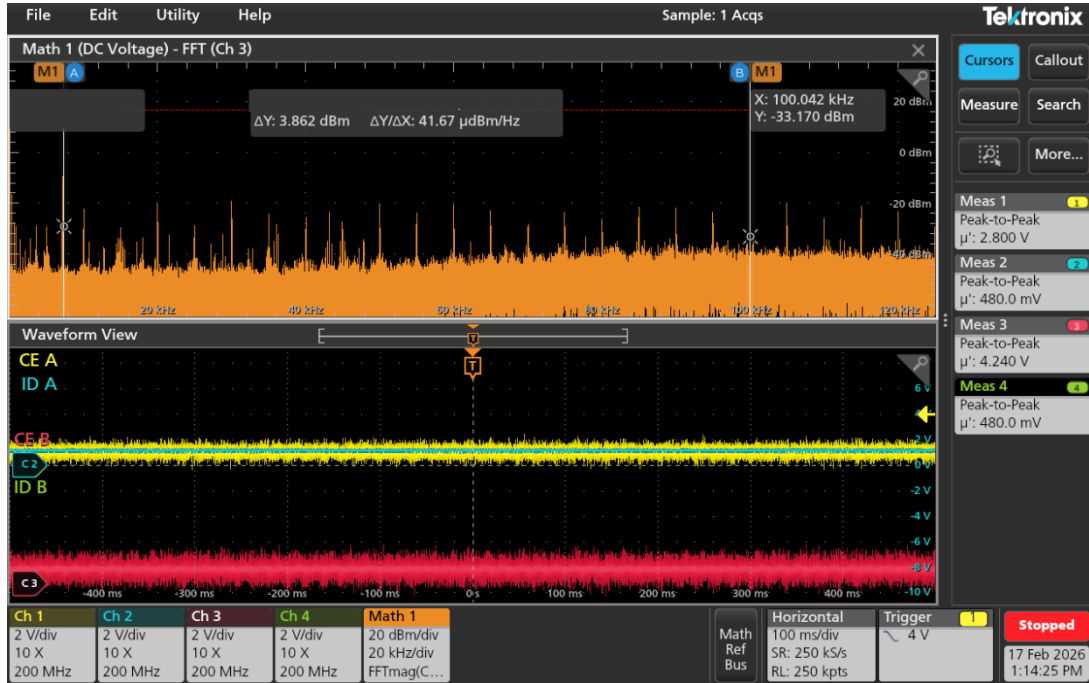
Figure 9 FFT of the CE signal.
