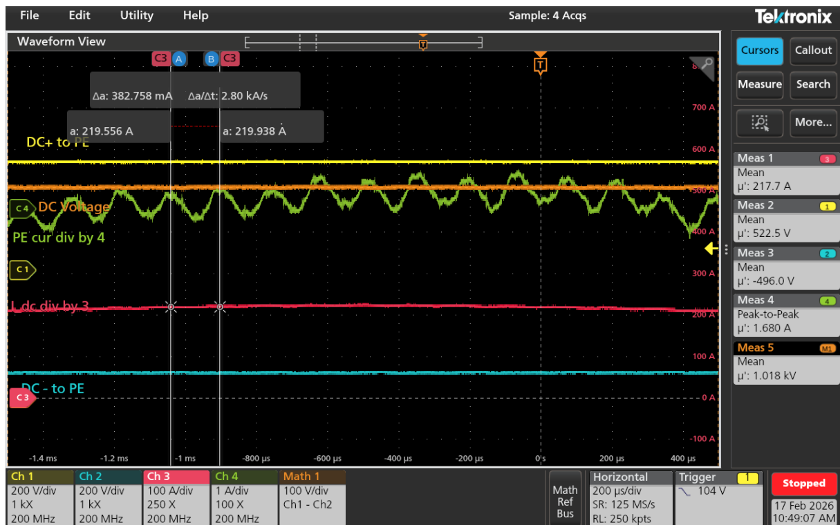
Figure 23 Main noise frequency on the PE current, that is the two times the power converter switching frequency.
