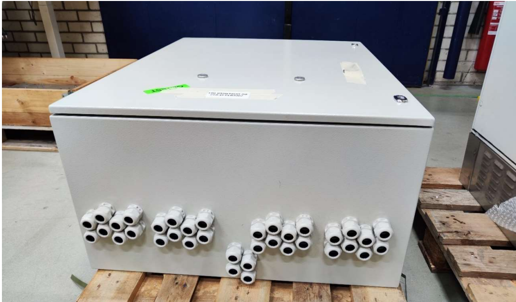
Figure 10 external cabinet of the DC outlet dispenser (glands grouped per DC-field, to be connected with dedicated tooling due to small mutual distances).
