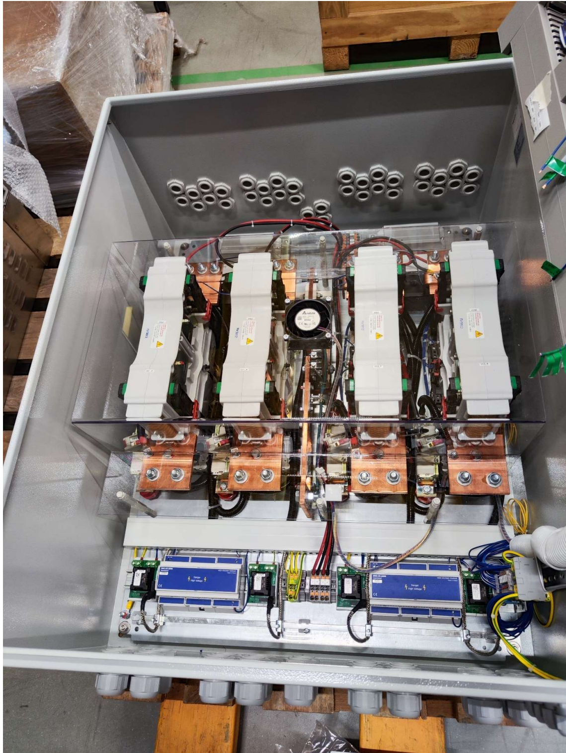
Figure 12 internal power section of the DC outlet dispenser
