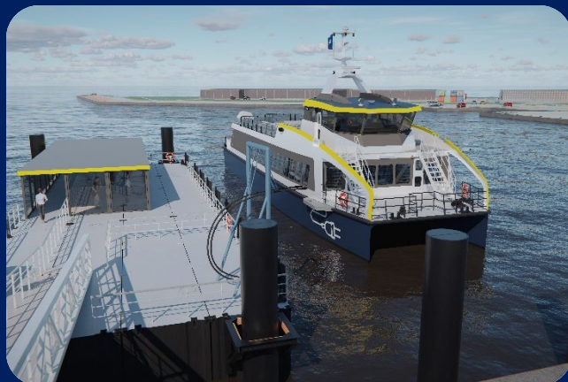
Computer animation of the battery-electric catamaran with ponton and charging station
