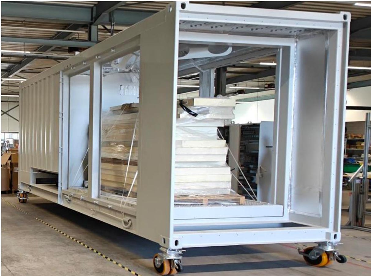
Figure 17 gross container without doors showing inserted and to-be-inserted insulation panels.
