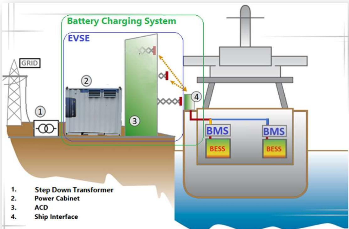
Figure 1 System Representation and Main Functional Blocks Identification
