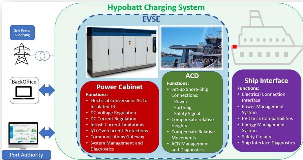
Figure 2 Functional Blocks Identification and main internal functions
