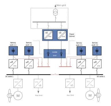
*Figure 7. Topology with direct (fast) battery charging, can be used for primary AC and DC systems (bustie is optional).*
