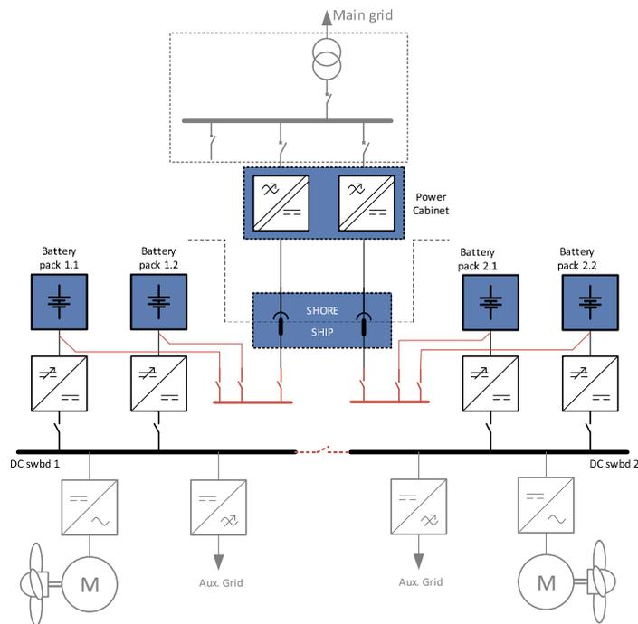
Figure 7. Topology with direct (fast) battery charging, can be used for primary AC and DC systems (bus-tie is optional).
