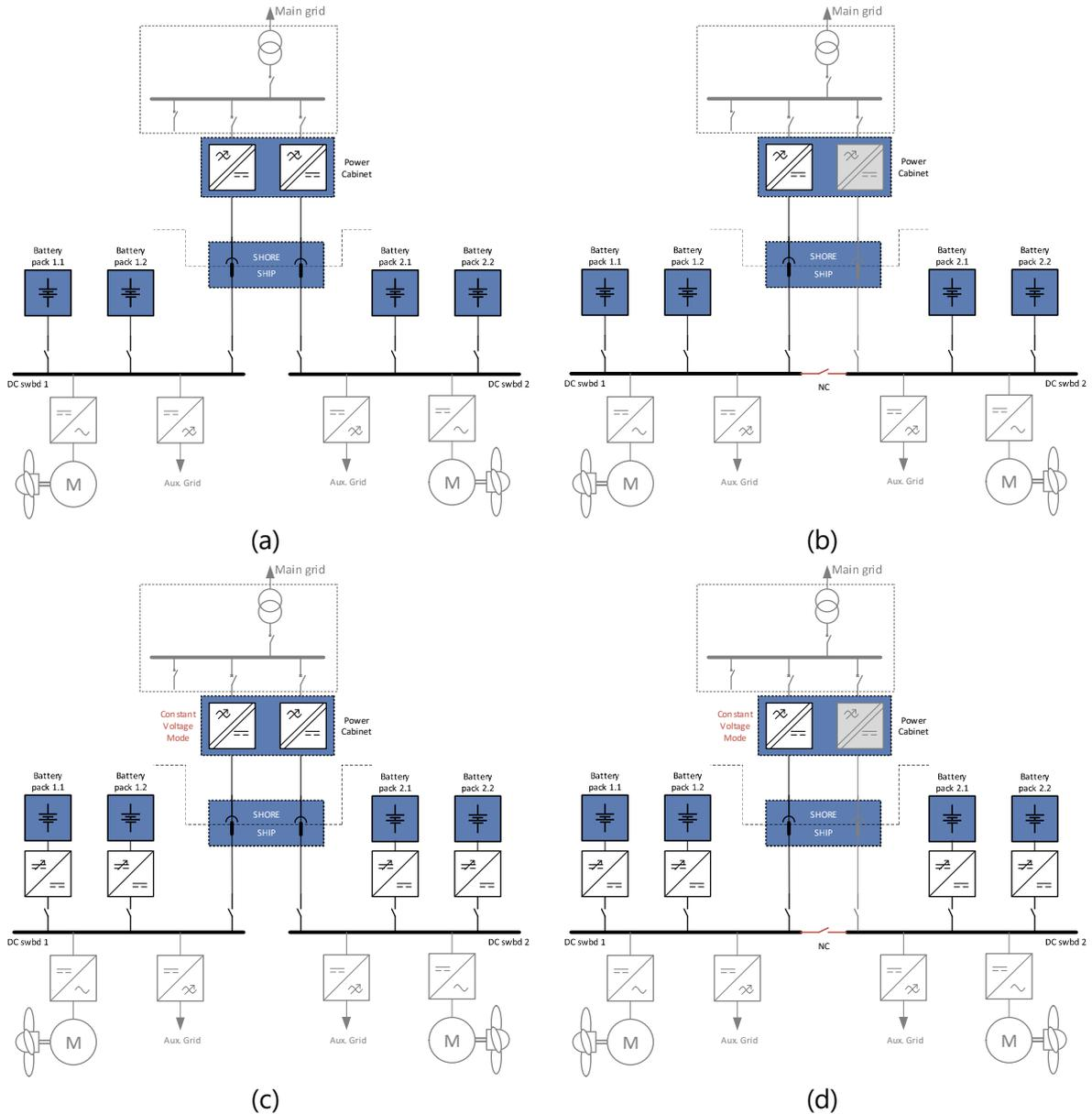
Figure 6. Suggested topologies for electric ship chargers, with (a) and (b) direct battery charging via DC-bus, and (c) and (d) DC-shore supply with onboard chargers.
