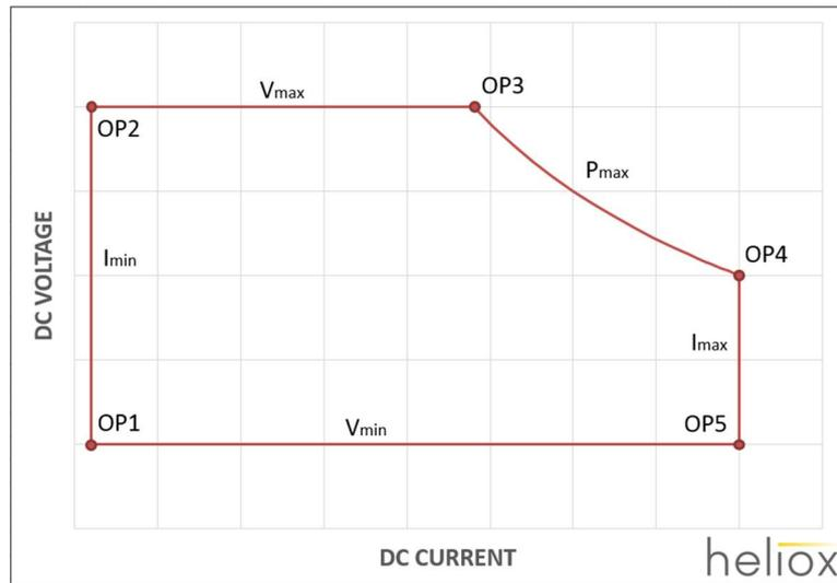
Figure 5 Envelope of DC power as a function of DC voltage vs. current with corner operating points (OP)
