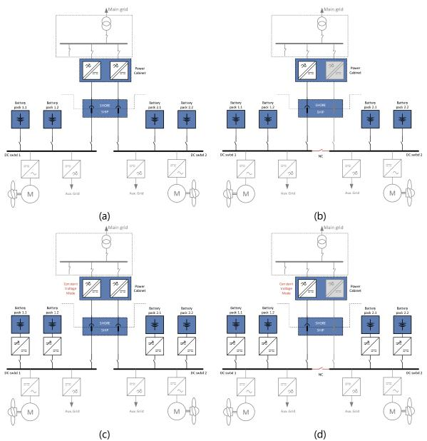
*Figure 6. Suggested topologies for electric ship chargers, with (a) and (b) direct battery charging via DCbus, and (c) and (d) DC-shore supply with onboard chargers.*
