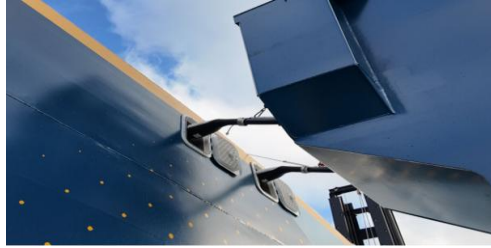
Figure 9 Same ship (dual) connection mated with manual connection (left) and temporary HYPOBATT ACD connection (right)
