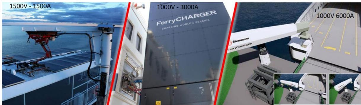
Figure 4: Typical ACD systems with from left to right: PANTO type, Tower type and BOW type
