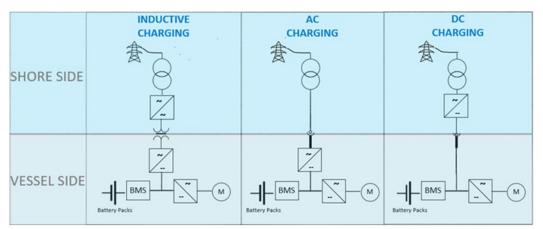
Figure 1. Conceptual charging solutions (Source: Stemmann Technik)
