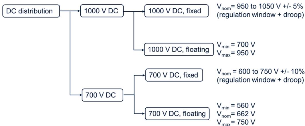
Figure 3. Vessel DC distribution topologies
