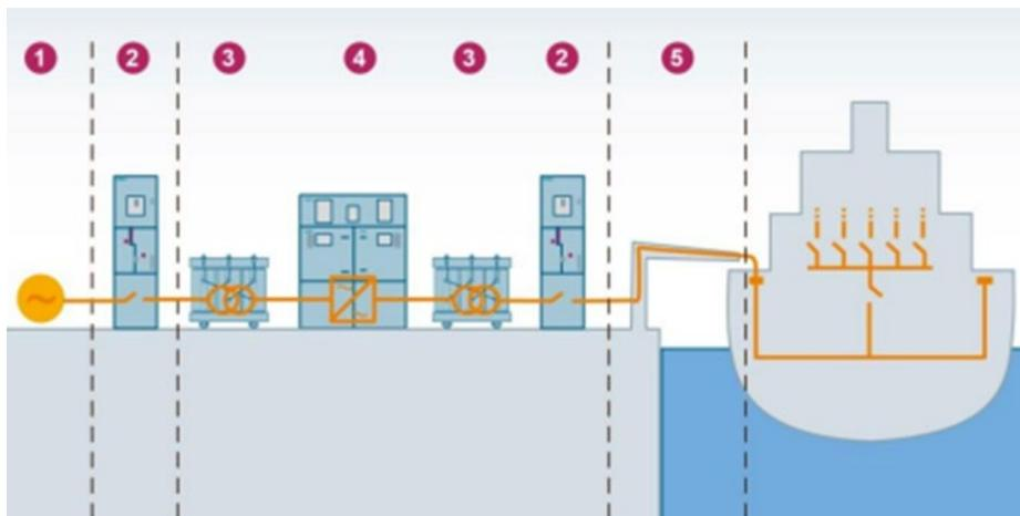
Figure 2. Typical OPS shore connection in Europe for berthed ships with 50/60 Hz frequency converter
