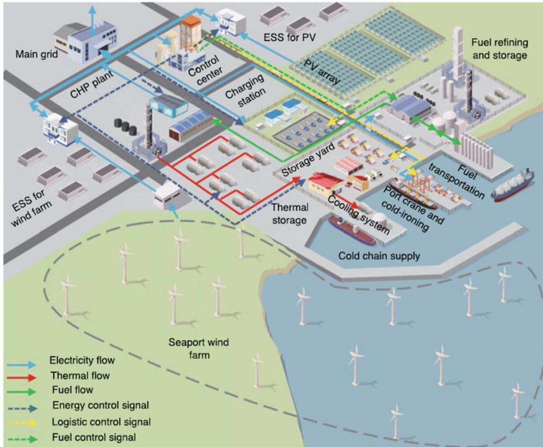
Figure 6: Energy flows and control in advanced shoreside energy management
