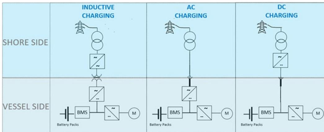
Figure 1. Conceptual charging solutions (Source: Stemmann Technik)
