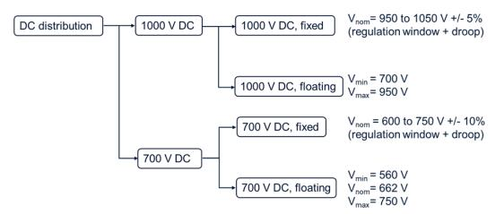
*Figure 3*. Vessel DC distribution topologies
